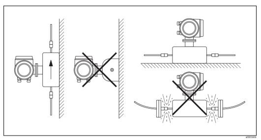
Fig. 9: Vertical and horizontal orientation (Promass A)
