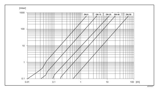
Fig. 57: Pressure loss diagram for water
