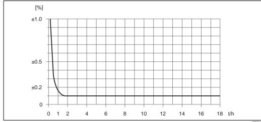
Fig. 44: Max. measured error in % o.r. (example: Promass H, DN 25)
