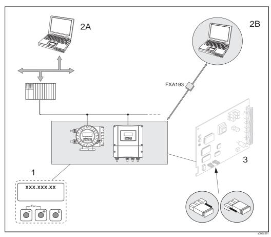
Fig. 26: FOUNDATION Fieldbus operating options
