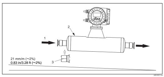
Fig. 12: Promass I: When lines are pitched in a specific direction and at a specific slope: as per hygienic guidelines (21 mm/m or approximatley 2%). Gravity can be used to achieve complete drainability.
