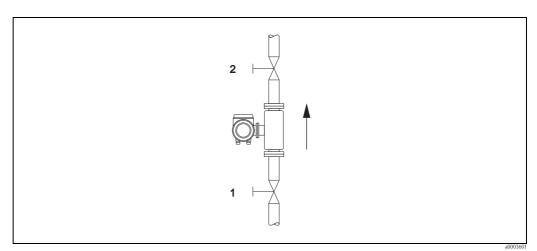
Fig. 36: Zero point adjustment and shutoff valves
