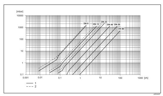
Fig. 52: Pressure loss diagram for water
