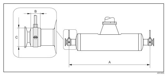
Fig. 14: Promass I, mounted with mounting clamp
