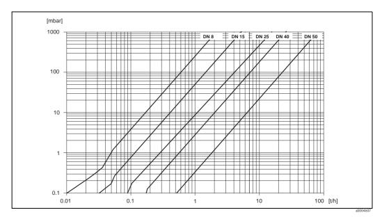
Fig. 55: Pressure loss diagram for water
