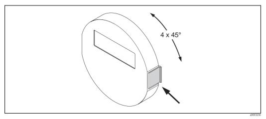
Fig. 21: Turning the local display (field housing)
