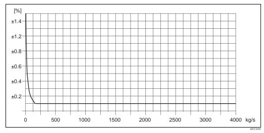
Fig. 50: Max. measured error in % o.r. (example: Promass 83X, DN 350)
