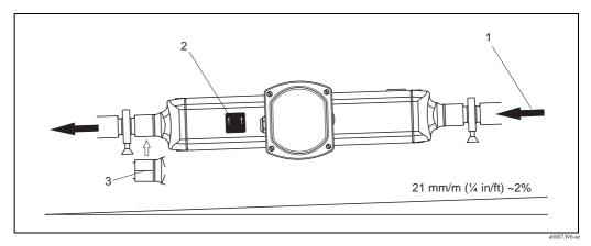
Fig. 11: Promass P: When lines are pitched in a specific direction and at a specific slope: as per hygienic guidelines (21 mm/m or approximatley 2%). Gravity can be used to achieve complete drainability.
