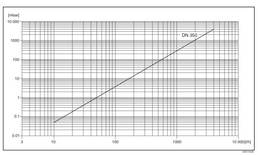
Fig. 59: Pressure loss diagram for water
