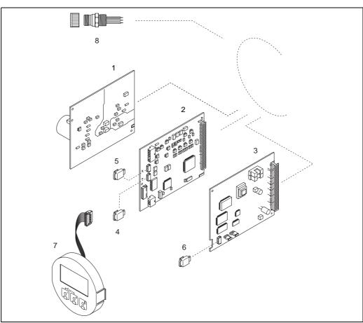
Fig. 37: Spare parts for transmitter (field and wall-mount housings)
