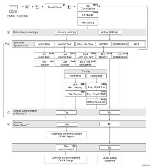
Fig. 32: Quick Setup "Commissioning" (only with local display)
