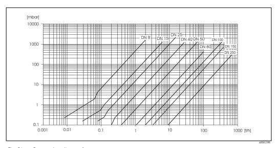
Fig. 51: Pressure loss diagram for water
