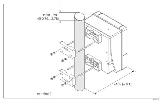
Fig. 20: Pipe mounting (wall-mount housing)
