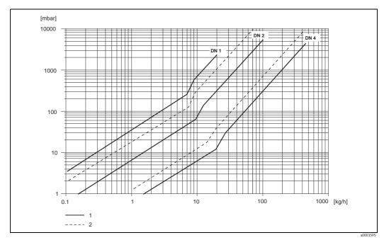
Fig. 54: Pressure loss diagram for water
