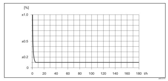
Fig. 47: Max. measured error in % o.r. (example DN 80)
