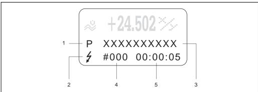
Fig. 30: Error messages on the display (example)
