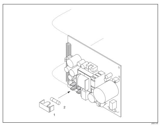
Fig. 40: Replacing the device fuse on the power unit board
