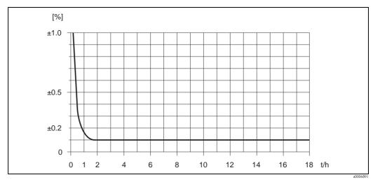
Fig. 48: Max. measured error in % o.r. (example: Promass P, DN 25)
