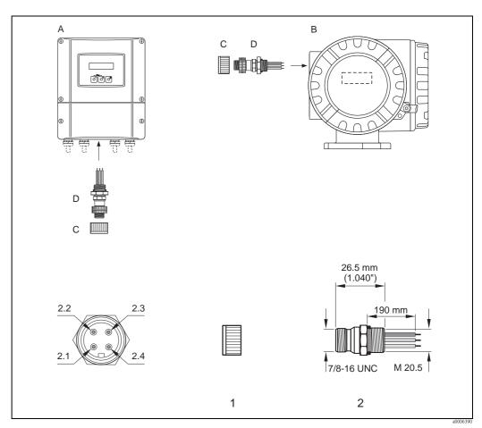
Fig. 24: Connector for connecting to the FOUNDATION Fieldbus
