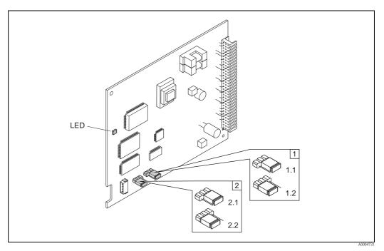
Fig. 31: Hardware configuration (I/O board)
