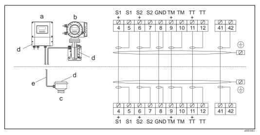
Fig. 22: Connecting the remote version
