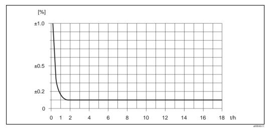
Fig. 49: Max. measured error in % o.r. (example: Promass S, DN 25)
