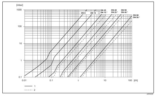
Fig. 56: Pressure loss diagram for water
