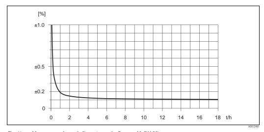
Fig. 46: Max. measured error in % o.r. (example: Promass M, DN 25)
