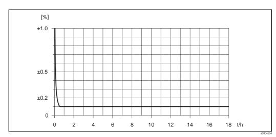
Fig. 43: Max. measured error in % o.r. (example: Promass F, DN 25)
