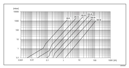
Fig. 53: Pressure loss diagram for water
