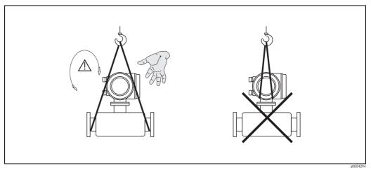
*Fig. 4:* Instructions for transporting sensors with > DN 40 (> 1½")
