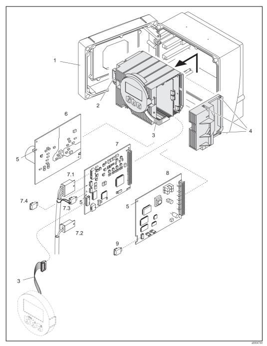
Fig. 39: Wall-mount housing: removing and installing electronics boards
