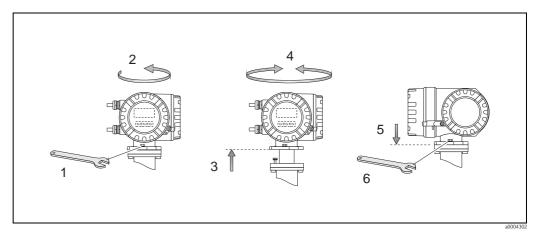
Fig. 16: Turning the transmitter housing (aluminum field housing)
