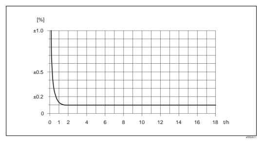
Fig. 45: Max. measured error in % o.r. (example: Promass I, DN 25)
