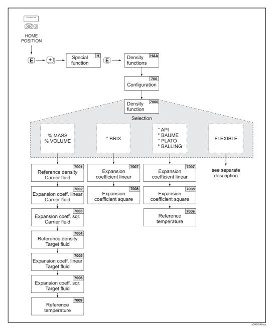
Fig. 35: Selecting and configuring different density functions in the function matrix
