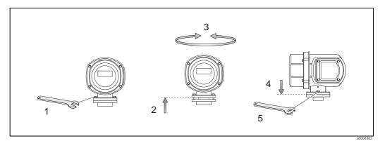
Fig. 17: Turning the transmitter housing (stainless steel field housing)
