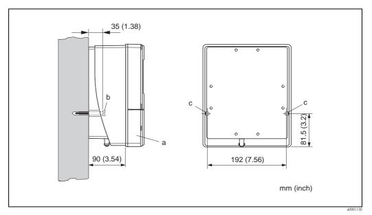
Fig. 18: Mounted directly on the wall
