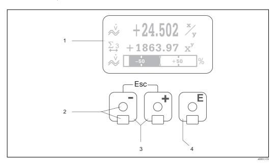
Fig. 27: Display and operating elements
