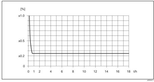
Fig. 42: Max. measured error in % o.r. (example: Promass E, DN 25)
