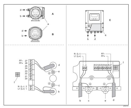
Fig. 23: Connecting the transmitter; cable cross-section: max. 2.5 mm<sup>2</sup>
