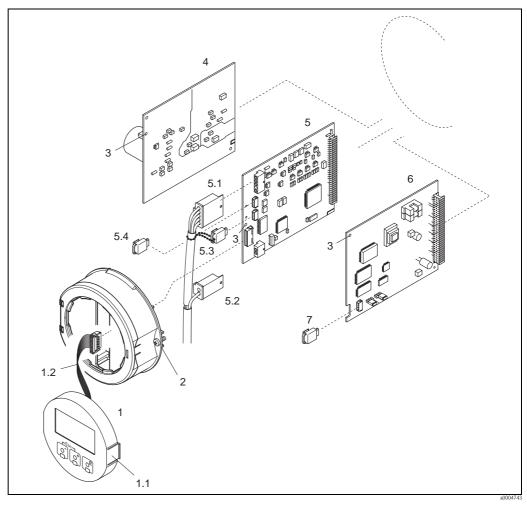
Fig. 38: Field housing: removing and installing electronics boards
