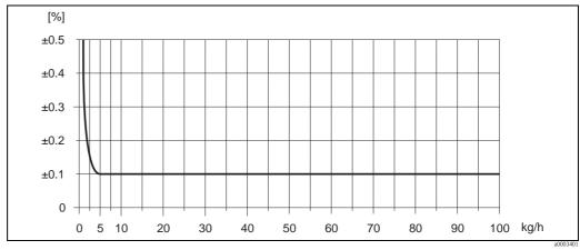
Fig. 41: Max. measured error in % o.r. (example: Promass A, DN 2)
