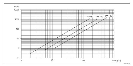
Fig. 58: Pressure loss diagram for water
